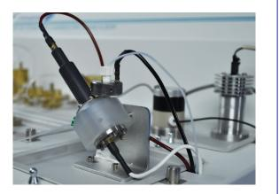
The FS3700 measures total cyanide by a UV digestion, gas diffusion technique coupled with amperometric detection in accordance with ASTM Method D7511-12.
